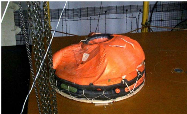
Figure 2. Life raft during wind test (research report, 2000)[15]
